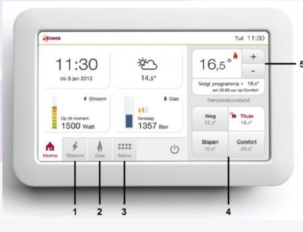
Figure 1: The Toon smart thermostat tablet device. With (1) historical electricity consumption; (2) historical gas consumption; (3) programme customisation, social comparison, usage pricing and baseline usage; (4) thermostat programme category; (5) manual thermostat adjustment. © energyfestival.eu.
